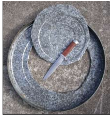
One of the first tests that I put the Rock Creek Eland to was cutting a circular hole out of an old garbage can lid because combat troops often use their knives to cut holes in similar thickness metal sheeting. While the edge certainly lost most of its keenness, there was no damage done to the knife.
